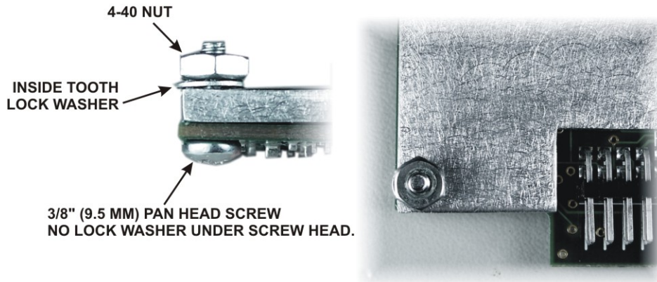
Figure 71 Stiffener Fastener on KSYN3 Board.
