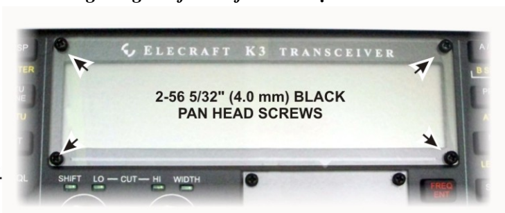
Figure 46. Installing LCD Cover.
