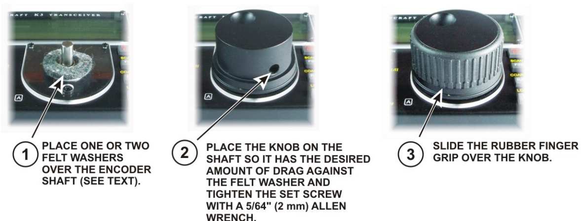
Figure 49. Mounting the VFO A Tuning Knob.
