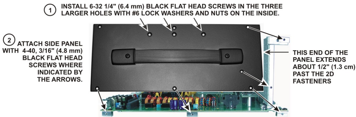
Figure 16. Mounting Left Side Panel.
