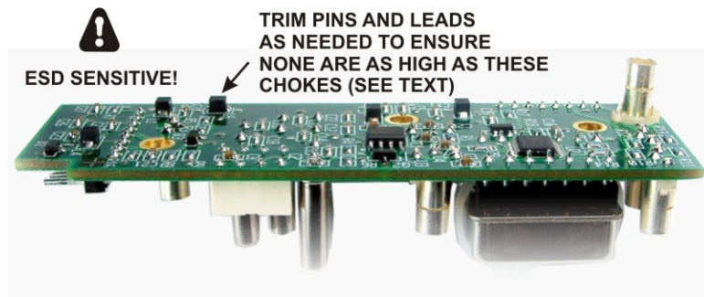
Figure 69. Checking Lead Lengths on KREF3 Board.
